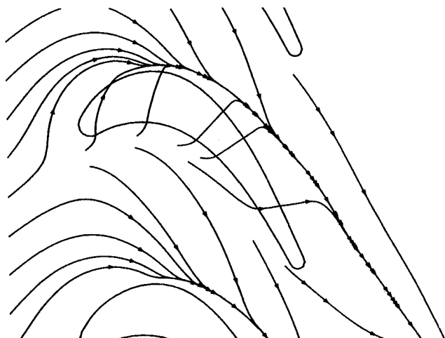
Fig. 5 Limiting streamline at near tip endwall.
